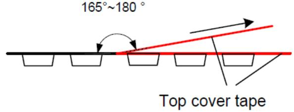
Peel-off speed: 300mm/min.
