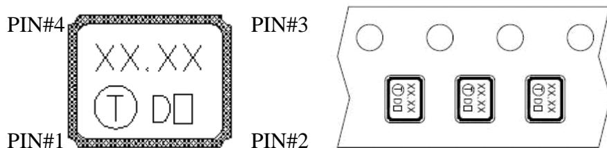
The inner vision of PIN#1, PIN#4 side is XTAL blank mounting pad.
